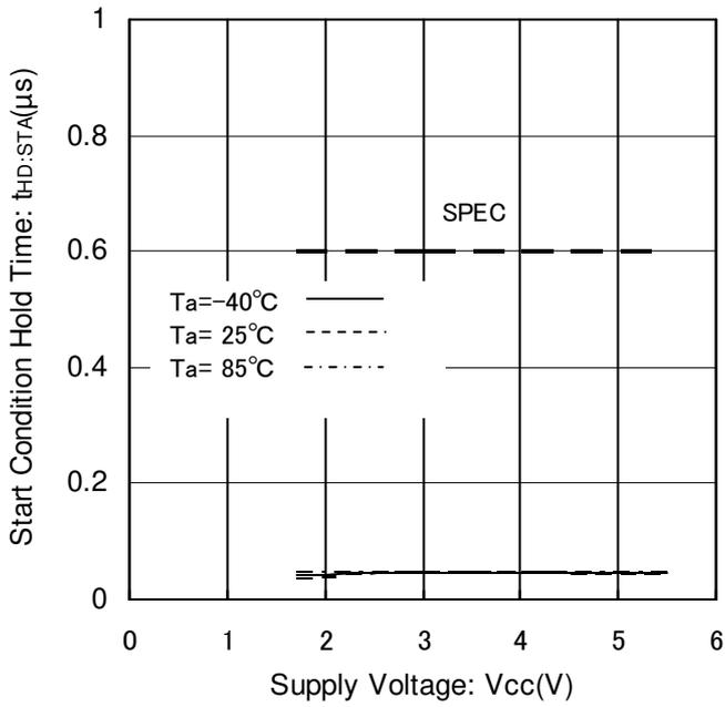
Figure 16. Start Condition Hold Time vs Supply Voltage
