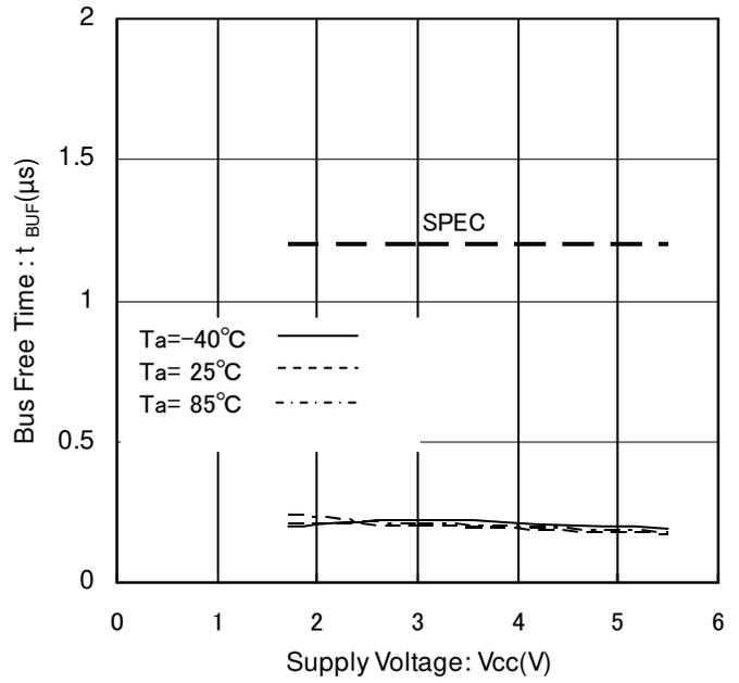
Figure 25. Bus Free Time vs Supply Voltage
