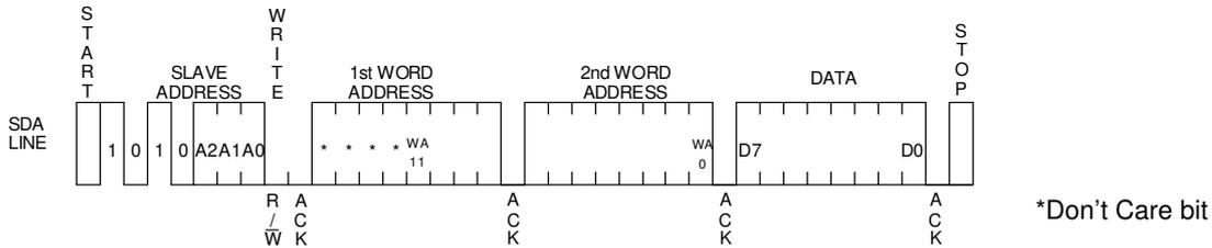
Figure 35. Byte Write Cycle
