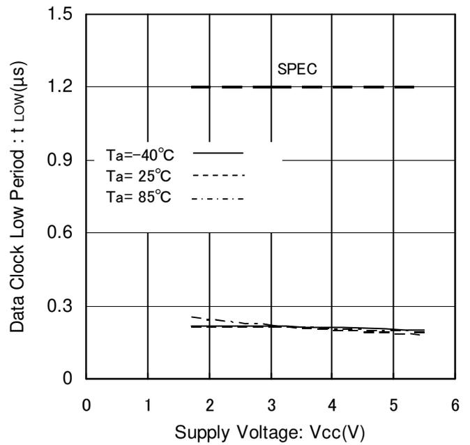
Figure 15. Data Clock Low Period vs Supply Voltage
