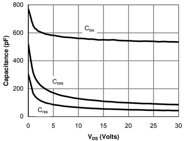
Figure 8: Capacitance Characteristics
