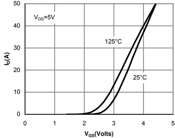
Figure 2: Transfer Characteristics
