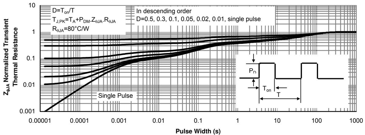
Figure 11: Normalized Maximum Transient Thermal Impedance (Note E)
