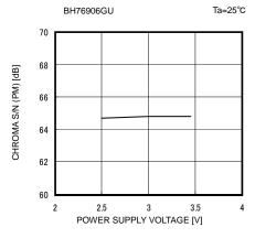
Fig. 51 C PM S/N vs Supply Voltage
