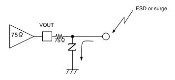
Fig.59 Using Externally Attached Varistor
