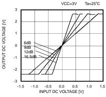
Fig. 38 DC I/O Characteristic
