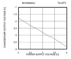
Fig. 41 Charge Pump Output Voltage vs Supply Voltage
