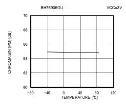
Fig. 52 C PM S/N vs Ambient Temperature
