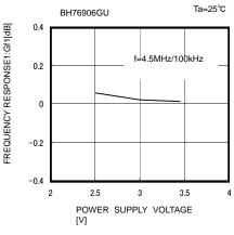
Fig. 28 Frequency Characteristic 1 vs Supply Voltage
