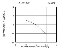
Fig. 43 Differential Phase vs Supply Voltage
