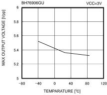
Fig. 37 Max. Output Level vs Ambient Temperature
