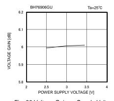
Fig. 26 Voltage Gain vs Supply Voltage
