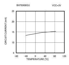
Fig. 17 Circuit Current vs Ambient Temperature
