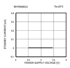
Fig. 18 Standby Circuit Current vs Supply Voltage
