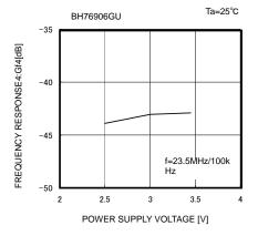
Fig. 34 Frequency Characteristic4 vs Supply Voltage
