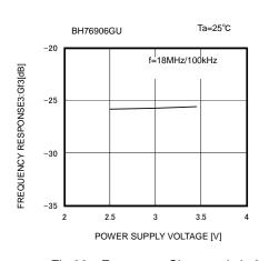
Fig.32 Frequency Characteristic 3 vs Supply Voltage
