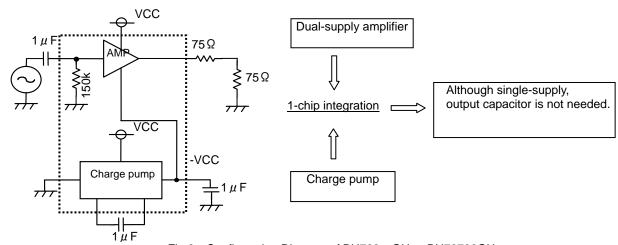
Fig.6 Configuration Diagram of BH769xxGU or BH76706GU
