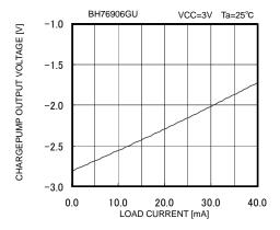
Fig. 42 Charge Pump Load Regulation
