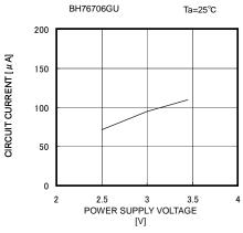
Fig. 20 GND Mode Circuit Current vs Supply Voltage
