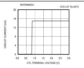
Fig. 55 Control Pin Characteristic
