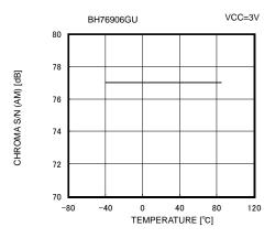
Fig. 50 C AM S/N vs Ambient Temperature
