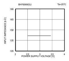
Fig. 53 Input Impedance vs Supply Voltage
