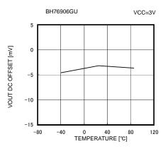
Fig. 23 VOUT Pin Output DC Offset vs Ambient Temperature
