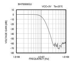
Fig. 24 Frequency Characteristic
