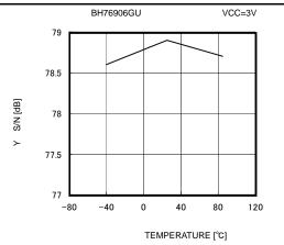
Fig.48 Y S/N vs Ambient Temperature
