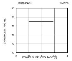
Fig. 49 C AM S/N vs Supply Voltage
