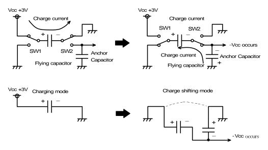
Fig.5 Principles of Charge Pump Circuit
