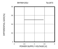
Fig. 45 Differential Gain vs Supply Voltage
