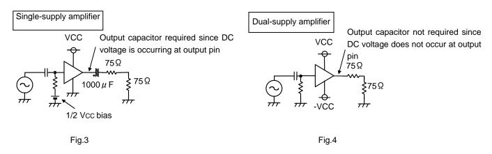
For an amplifier operated from a single power supply (single-supply), since the operating point has a potential of approximately 1/2 Vcc, a coupling capacitor is required for preventing direct current in the output. Moreover, since the load resistance is 150  $\Omega$  (75  $\Omega$  + 75  $\Omega$ ) for the video driver, the capacity of the coupling capacitor must be on the order of 1000  $\mu$ F if you take into account the low band passband. (Fig.3)
