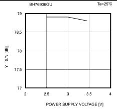
Fig. 47 Y S/N vs Supply Voltage
