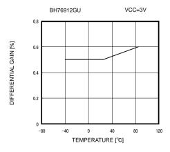
Fig. 46 Differential Gain vs Ambient Temperature
