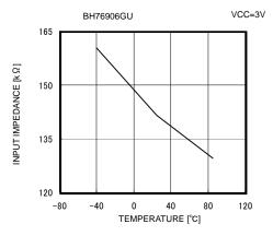
Fig. 54 Input Impedance vs Ambient Temperature
