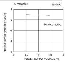
Fig. 30 Frequency Characteristic 2 vs Supply Voltage
