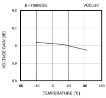
Fig. 27 Voltage Gainvs Ambient Temperature
