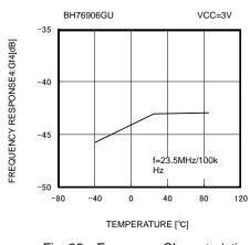
Fig. 35 Frequency Characteristic 4 vs Ambient Temperature
