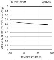
Fig. 32 Maximum output level vs. Temperature
