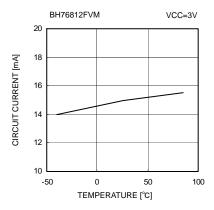
Fig. 18 Circuit current vs. Temperature
