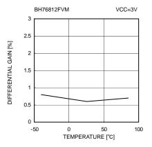
Fig. 41 Differential gain vs. Temperature
