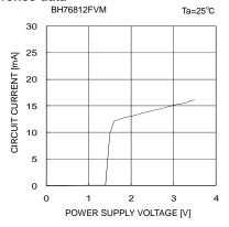
Fig. 16 Circuit current vs. Supply voltage
