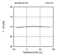
Fig.43 S/N(Y) vs. Temperature
