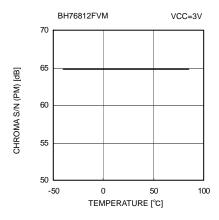
Fig. 47 S/N(C-PM) vs. Temperature
