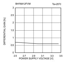
Fig. 40 Differential gain vs. Supply voltage
