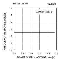
Fig. 27 Frequency response 2 vs. Supply voltage
