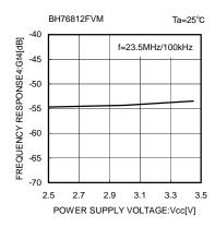
Fig.29 Frequency response 4 vs. Supply voltage
