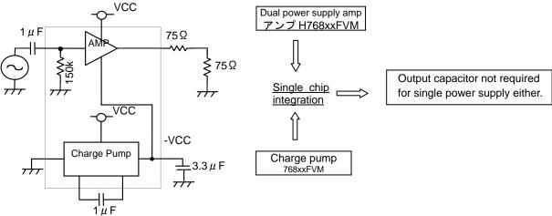
Fig. 6 BH768xxFVM Configuration Diagram
