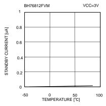
Fig. 19 Circuit Current (Standby) vs. Temperature
