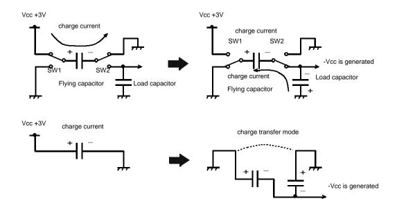
Fig. 5 Principles of Charge Pump Circuit
