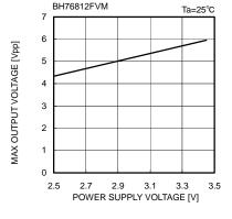
Fig. 31 Maximum output voltage level vs. Supply voltage
