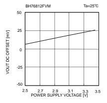
Fig. 20 Vout DC offset voltage vs. Supply voltage
