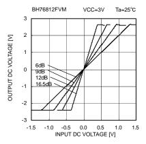
Fig. 33 Output DC voltage - Input DC voltage
