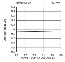
Fig. 23 Voltage gain vs. Supply voltage
