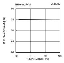
Fig. 45 S/N(C-AM) vs. Temperature
