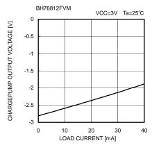
Fig. 37 Charge pump load regulation
