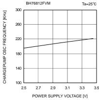
Fig. 34 Charge pump oscillation frequency vs. Supply voltage
