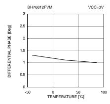
Fig. 39 Differential phase vs. Temperature
