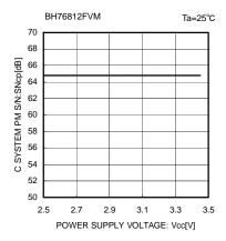
Fig. 46 S/N(C-PM) vs. Supply Voltage
