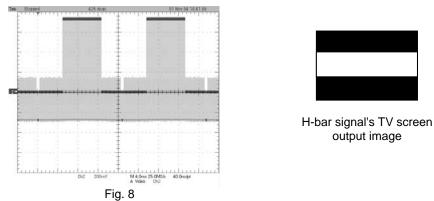
b) BH768xxFVM output (input = 1.0 μF, TG-7/1 output, H-bar)
