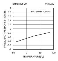
Fig. 26 Frequency response 1 vs. Temperature
