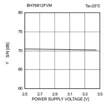
Fig. 42 S/N(Y) vs. Supply Voltage
