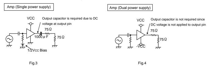
When the amplifier operates using single voltage power supply, the operating potential point is approximately 1/2 Vcc. Therefore, a coupling capacitor is required to prevent DC output. For the video driver, the load resistance is 150  $\Omega$  (75  $\Omega$  + 75  $\Omega$ ). Therefore, the coupling capacitor should be about 1000  $\mu$ F when a low bandwidth for transmission is considered. (See Figure 3.)
