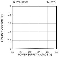
Fig. 17 Circuit Current (Standby) vs. Supply Voltage
