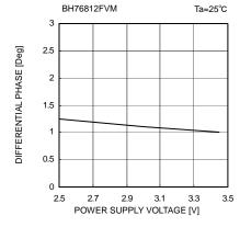
Fig. 38 Differential phase vs. Supply voltage
