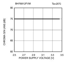
Fig. 44 S/N(C-AM) vs. Supply Voltage
