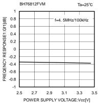
Fig. 25 Frequency response 1 vs. Supply voltage
