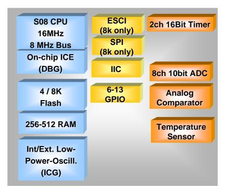
16 pin QFN, TSSOP, PDIP 8 pin DFN, SOIC, PDIP MC9S08QG4CPAE .... \$0.89/1kpcs
