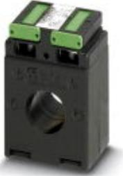
Bus-bar current transformer, 200 A AC primary current; 5 A AC secondary current; accuracy class 1; 5 VA rated power
