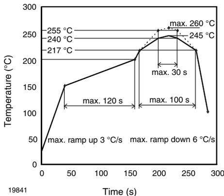
Fig. 6 - Lead (Pb)-free Reflow Solder Profile acc. J-STD-020
