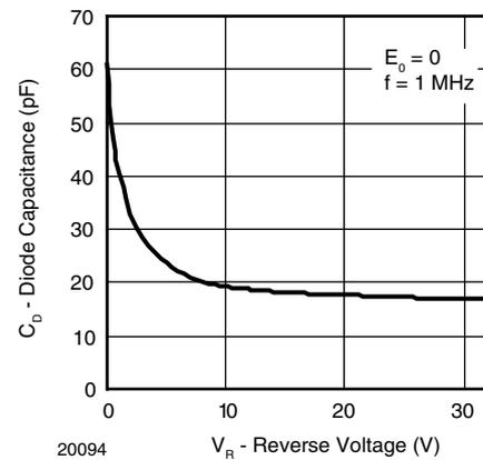
Fig. 3 - Diode Capacitance vs. Reverse Voltage
