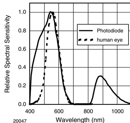
Fig. 4 - Relative Spectral Sensitivity vs. Wavelength
