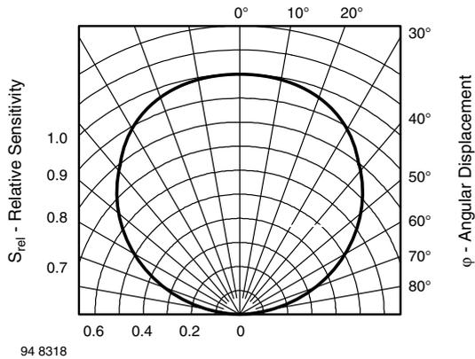
Fig. 5 - Relative Radiant Sensitivity vs. Angular Displacement
