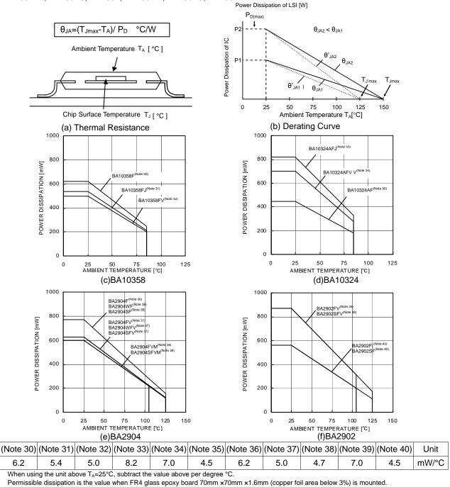
Figure 102. Thermal resistance and derating
