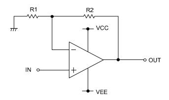
For non-inverting amplifier, IN is amplified by voltage gain decided R1 and R2, and phase is same with IN. OUT is shown next formula.  $OUT = (1+R2/R1) \cdot IN$
