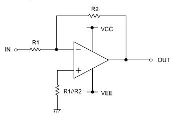
For inverting amplifier, IN is amplified by voltage gain decided R1 and R2, and phase reversed voltage is output.
