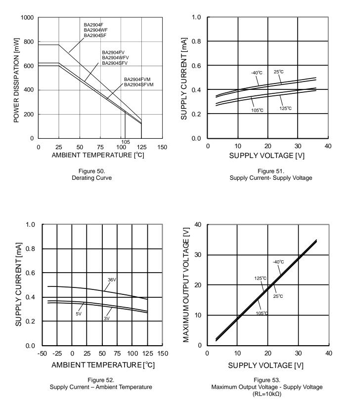
(\*) The above data is measurement value of typical sample, it is not guaranteed. BA2904, BA2904W : -40°C to  $+125^{\circ}$ C BA2904S : -40°C to  $+105^{\circ}$ C
