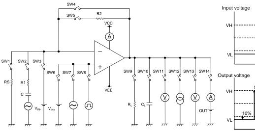
Figure 99. Test Circuit 2 (each Op-Amp)
