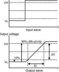
Figure 100. Slew Rate Input Waveform
