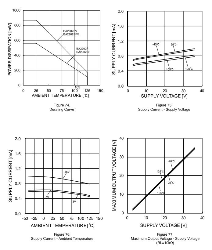
(\*) The above data is measurement value of typical sample, it is not guaranteed. BA2902 : -40°C to +125°C BA2902S : -40°C to +105°C
