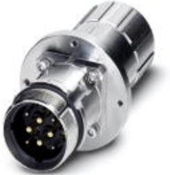
Pin/socket, panel feed-through, straight, M40, M40, Number of positions: 4+3+PE, Type of contact: Socket, Crimp connection, Axial O-ring, 4xM4, Shielded: Yes, Cable cross section: 0 mm...0 mm
