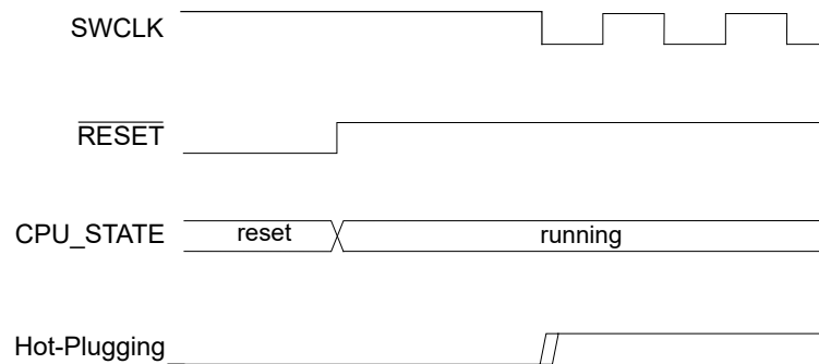
Figure 16-3. Hot-Plugging Detection Timing Diagram
