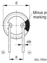
Minus pole The series B41898 has no sleeve nor minus pole marking, the positive pole is marked on the aluminum case side instead.
