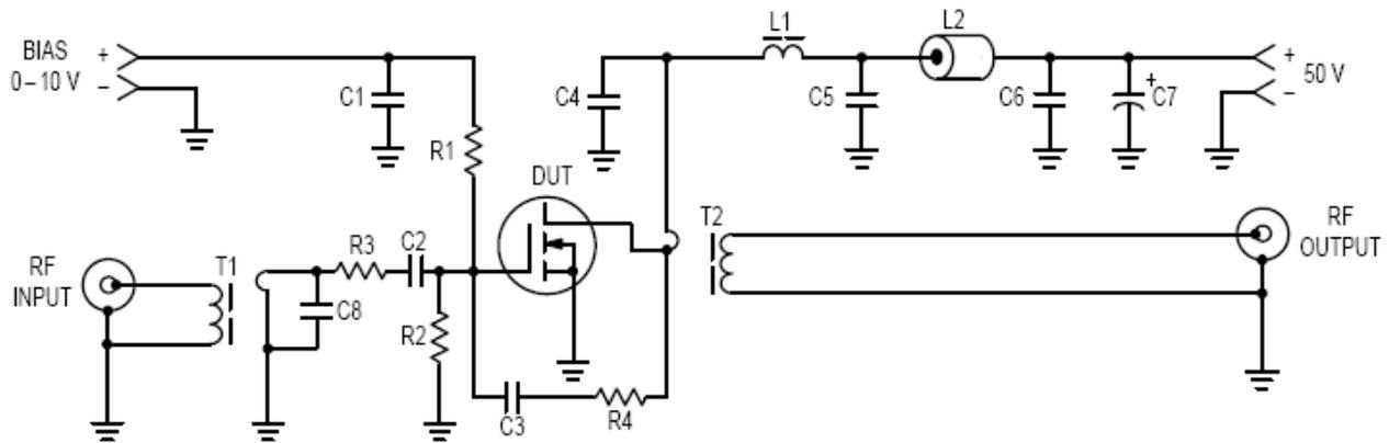
C1, C2, C3, C4, C5, C6 — 0.1  $\mu\text{F}$  Ceramic Chip or Equivalent
