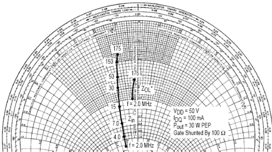
$Z_{OL}^*$  = Conjugate of the optimum load impedance into which the device output operates at a given output power, voltage and frequency.
