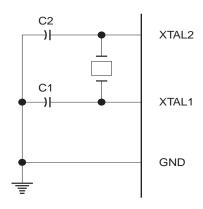
Note: C1, C2 = 30 pF  $\pm$ 10 pF for Crystals = 40 pF  $\pm$ 10 pF for Ceramic Resonators
