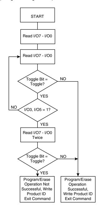
Note: 1. The system should recheck the toggle bit even if I/O5 = "1" because the toggle bit may stop toggling as I/O5 changes to "1".
