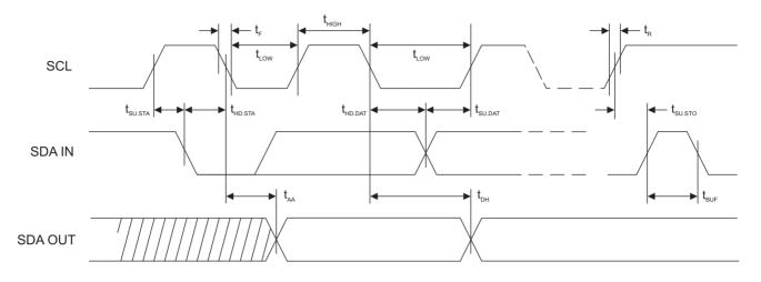
SCL: Serial Clock, SDA: Serial Data I/O
