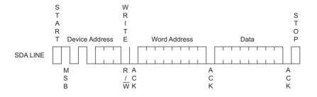
**Page Write:** The 16K EEPROM are capable of an 16-byte Page Write. A Page Write is initiated in the same way as a Byte Write, but the microcontroller does not send a Stop condition after the first data word is clocked in. Instead, after the EEPROM acknowledges receipt of the first data word, the microcontroller can transmit up to 15 data words. The EEPROM will respond with a zero after each data word received. The microcontroller must terminate the Page Write sequence with a Stop condition.
