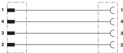
Contact assignment of M8 plugs/sockets
