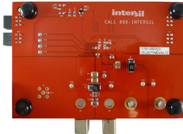
Figure 3. ISL8277MEVAL1Z Evaluation Board (Bottom Side)
