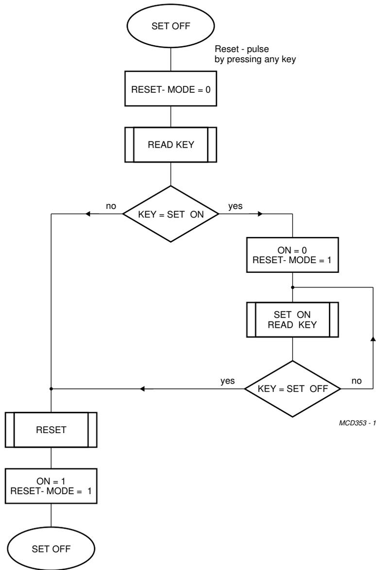
Fig.9 Flow chart for high end application.
