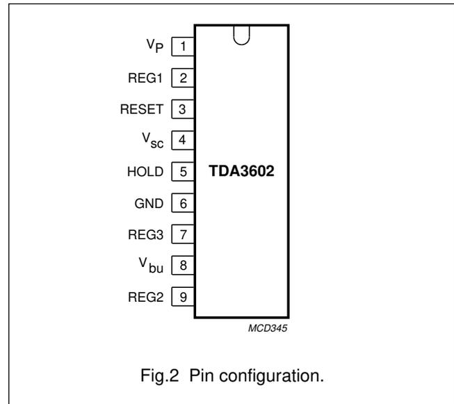
Fig.2 Pin configuration.
