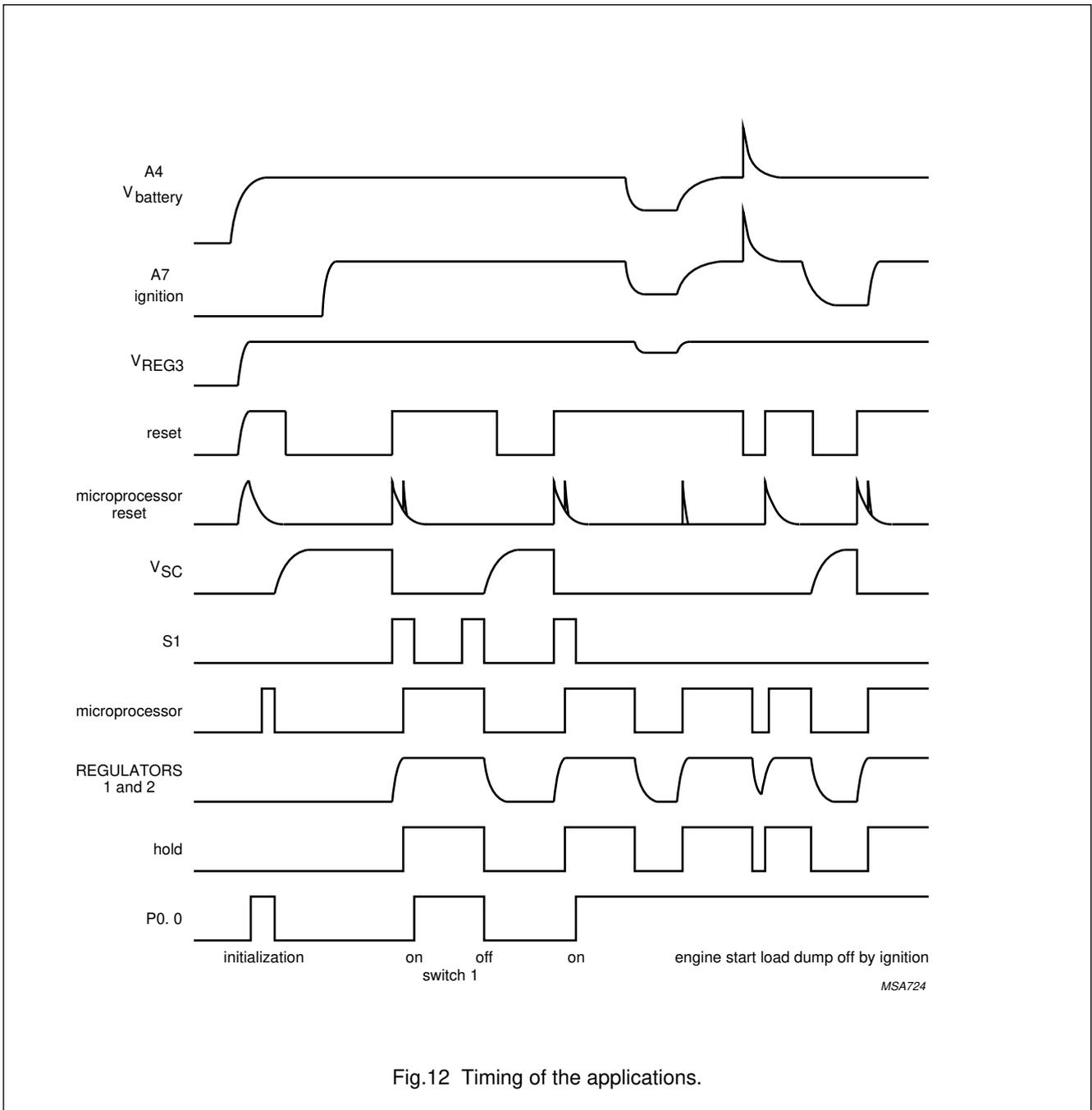
Fig.12 Timing of the applications.
