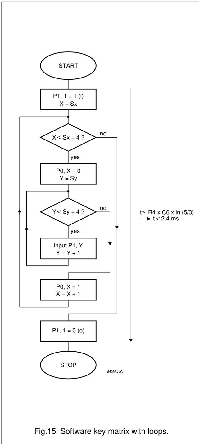
Fig.15 Software key matrix with loops.
