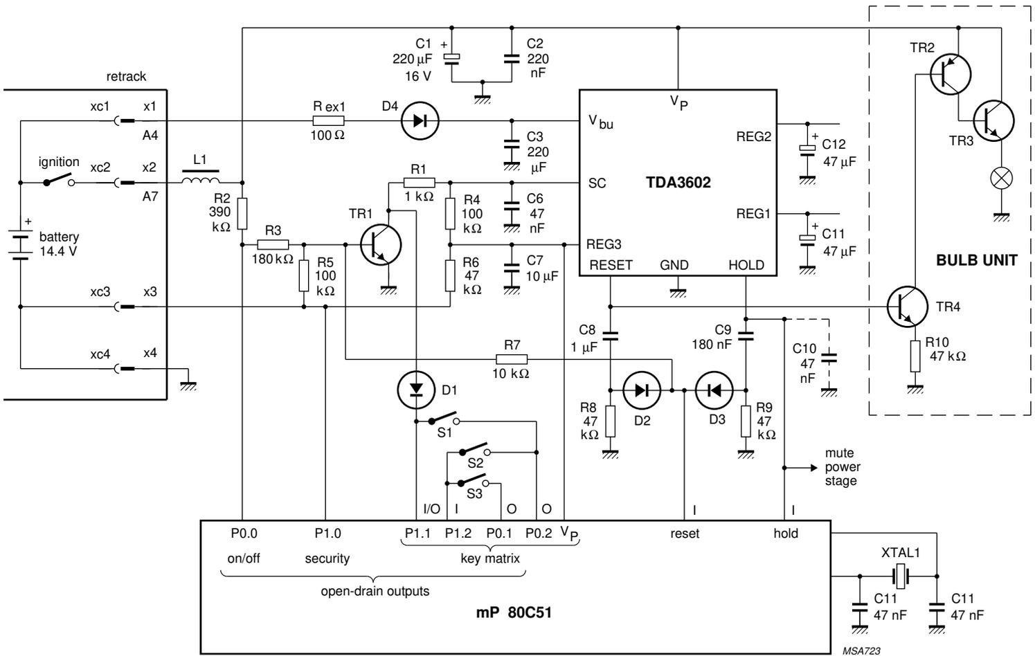
Fig.11 Application with all features of semi on/off logic.
