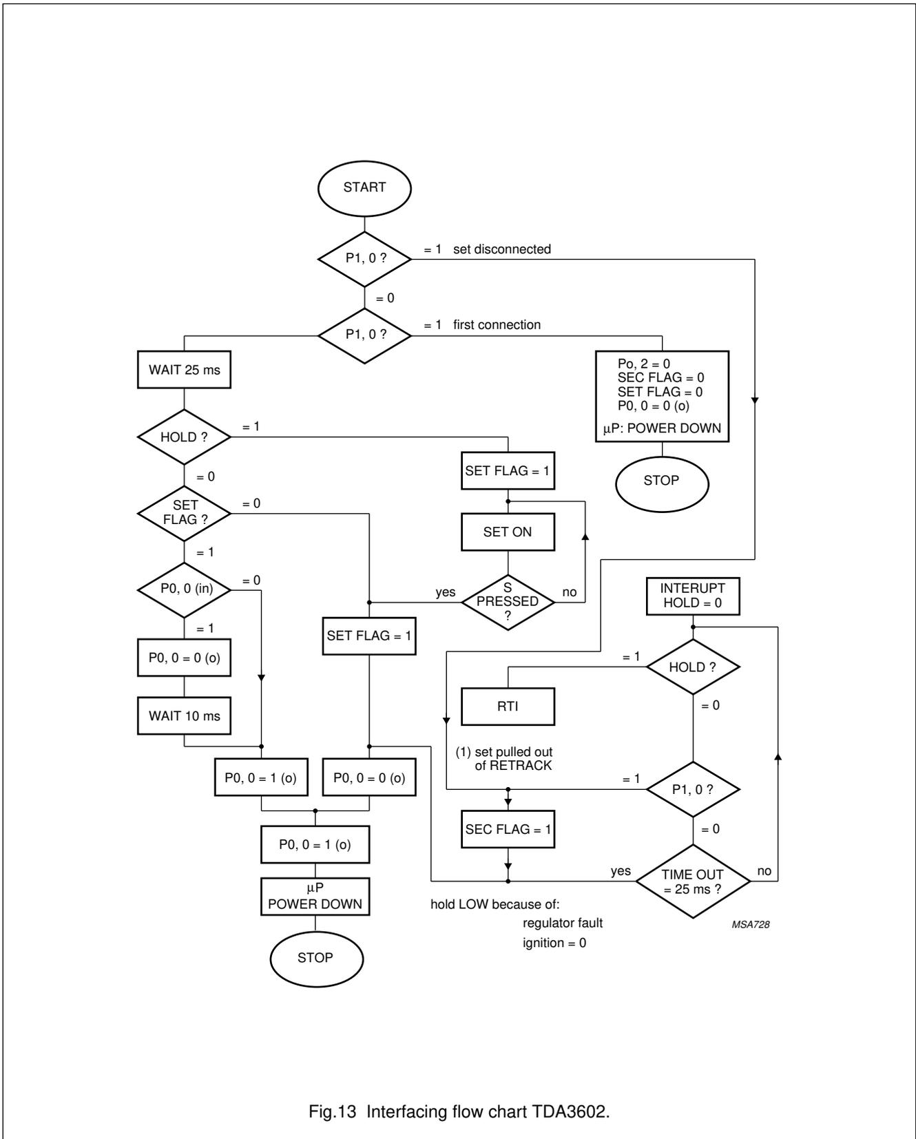
Fig.13 Interfacing flow chart TDA3602.
