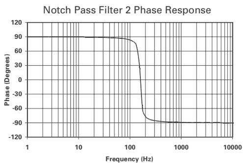
Typical responses for the circuit with component values shown in circuit diagram.
