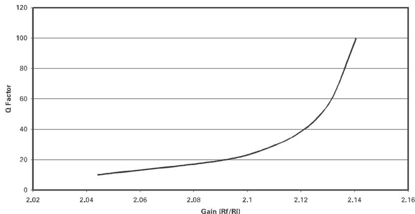
This diagram shows the exponential relationship between gain and Q Factor. (fo = 140 kHz)
