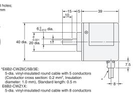
(Conductor cross section: 0.2 mm², Insulation diameter: 1.0 mm), Standard length: 0.5 m
