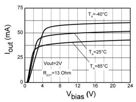
Fig. 12 Output Current vs. V<sub>bias</sub>
