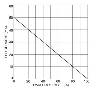
Fig. 17 Typical LED current response vs. PWM duty cycle for  $R_{\text{EXT}}$  = 13 $\Omega$  at 400Hz PWM frequency
