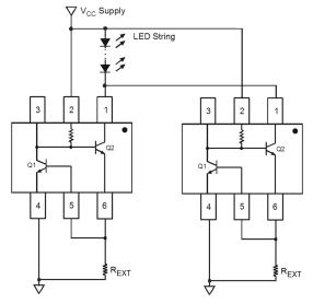
Fig. 15 Application Circuit for Increasing LED Current
