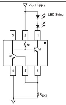
Fig. 14 Typical Application Circuit for Linear Mode Current Sink LED Driver
