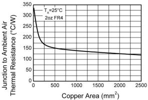
Fig. 4 Thermal Resistance vs. Area
