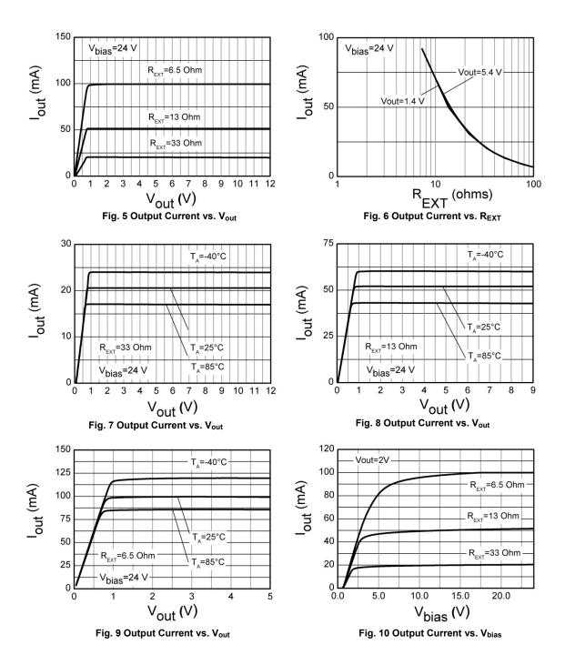
Note: 10. V<sub>out</sub> in the "Output current Vs V<sub>out</sub>" graphs limited by power dissipation in the device.
