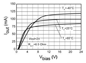
Fig. 13 Output Current vs. V<sub>bias</sub>
