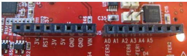
Figure 11. J4 and J5 Arduino Compatible Interface (Power and ADC)
