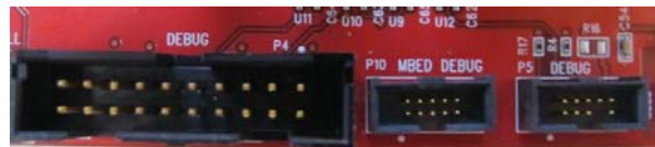
Figure 18. P4 and P5 Debug Connectors
