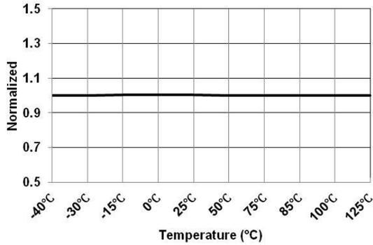
Figure 29. V<sub>IN</sub> UVP Disable Voltage at 9 V (V<sub>IN-UVP-H-9V</sub>) vs. Temperature
