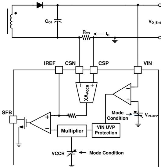
Figure 41. V<sub>IN</sub> Under-Voltage Protection Block
