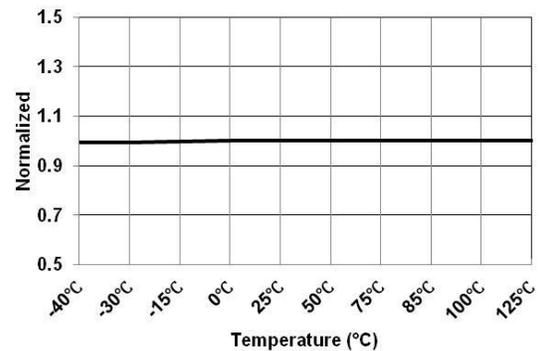
Figure 10. Reference Voltage for CC Regulation at Variable CC 7V Mode (V<sub>C CR-VR-7V</sub>) vs. Temperature
