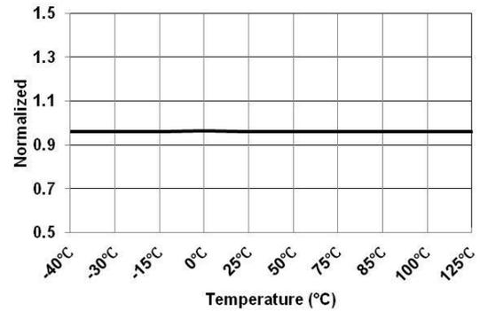
Figure 32. Charge Pump Disable Threshold Voltage (V<sub>IN-CP</sub>) vs. Temperature
