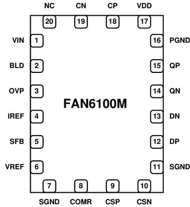
Figure 4. Pin Assignments
