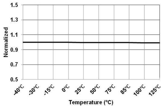
Figure 33. DP Low Level Threshold Voltage (V<sub>DPL</sub>) vs. Temperature
