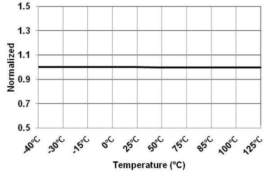
Figure 30. V<sub>IN</sub> UVP Enable Voltage at 12 V (V<sub>IN-UVP-L-12V</sub>) vs. Temperature
