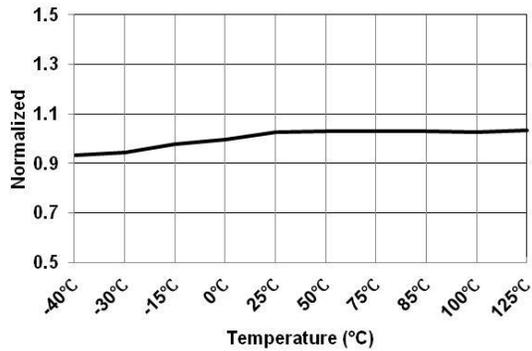
Figure 7. Operating Current Under 5 V (I<sub>IN-OP-LV</sub>) vs. Temperature
