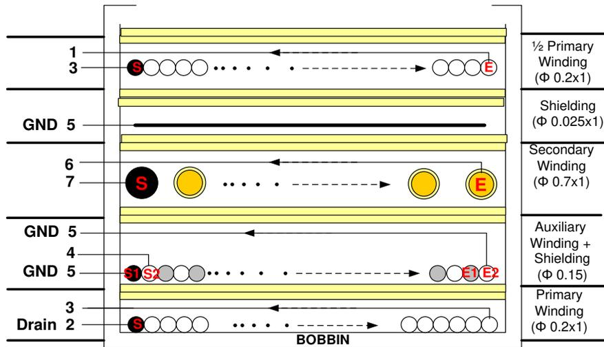
Figure 47. Transformer Diagram
