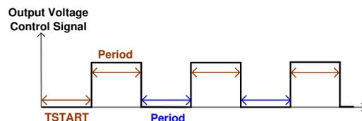
Figure 44. FCP-Single Communication Protocol Control Signal Waveform
