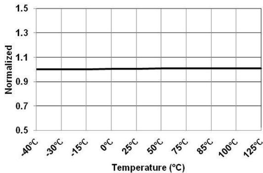
Figure 9. Reference Voltage for CC Regulation at Variable CC 5 V Mode (V<sub>C CR-VR-5V</sub>) vs. Temperature
