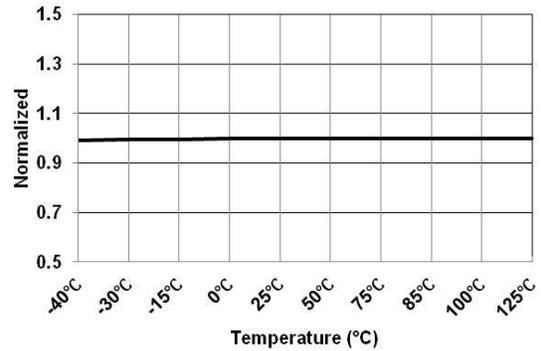
Figure 6. V<sub>DD</sub> Turn-Off Threshold Voltage (V<sub>DD-OFF</sub>) vs. Temperature
