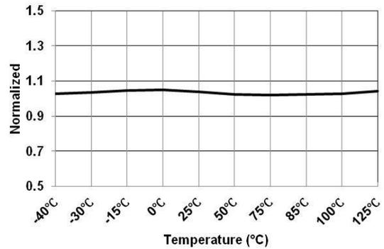
Figure 8. Operating Current Over 5 V (I<sub>IN-OP-HV</sub>) vs. Temperature
