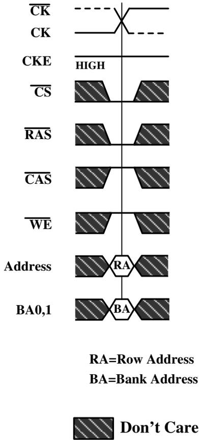
Figure 6.  $t_{RCD}$  and  $t_{RRD}$  Definition
