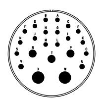
Note: Due to an automatic nomenclature system, numbers generated may not be sequential. Specification and Dimensions subject to chang Drawings illustrate normal insulator positioning Material Specification: Shell Material: Aluminium alloy Olive drab chromate coating over cadmium plating Shell Plating: Insulator Material: Neoprene Contact Material: Copper alloy Contact Plating: Hard silver
