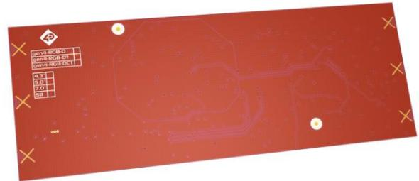
Where the Application PCB is shown to sit in Section 5.5, can house a small metal shield of the same size. This shield is used instead of, or underneath an Application PCB, to aid the on-board electronics in the prevention from potential RF or EMI signals.
