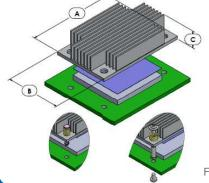
**NOTES:** 1) Dimension A is the length of the heat sink in the direction of the flow.
