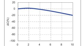
4) Bias TCC characteristics (Agilent 4284A, 1kHz, 1Vrms, 5Vdc)
