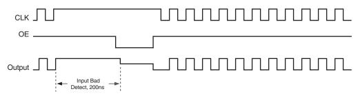
Figure 1F. OEx with Bad Input Timing Diagram
