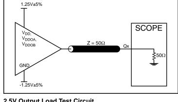
2.5V Output Load Test Circuit
