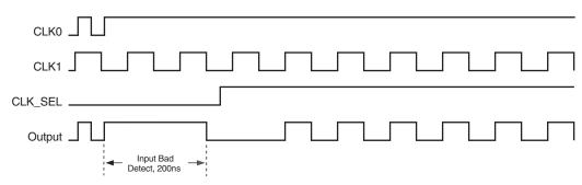
Figure 1D. CLK\_SEL with Bad Input Timing Diagram
