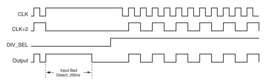
Figure 1E. DIV SELx with Bad Input Timing Diagram
