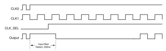
Figure 1G. CLK\_SEL with Bad Input Timing Diagram
