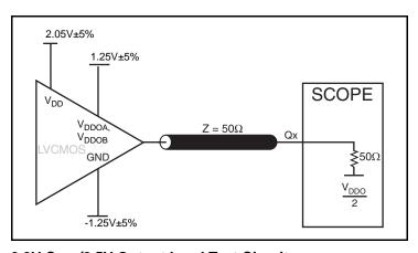
3.3V Core/2.5V Output Load Test Circuit
