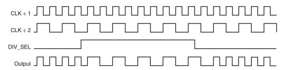
Figure 1B. DIV\_SELx Timing Diagram
