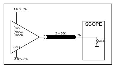
3.3V Output Load Test Circuit
