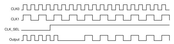
Figure 1A. CLK\_SEL Timing Diagram
