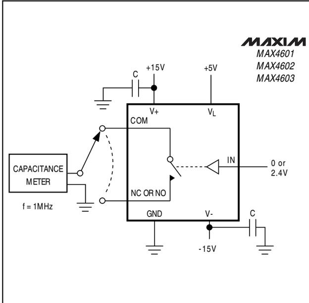
Figure 6. Switch Off-Capacitance Test Circuit
