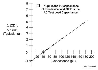
Figure 3. Typical Output Derating (Lumped Capacitive Load).
