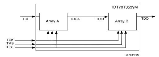
Figure 5. JTAG Configuration for IDT70T3539M
