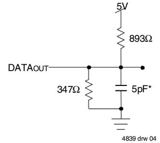
Figure 2. Output Test Load
