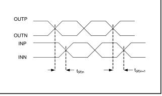
Figure 4: Static phase offset (from input to output)
