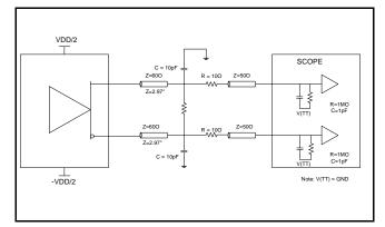
Figure 2: Output load test circuit
