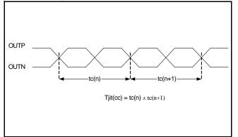
Figure 3: Cycle-cycle jitter
