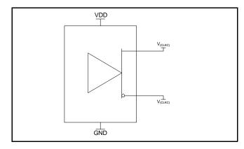
Figure 1: IBIS model output load
