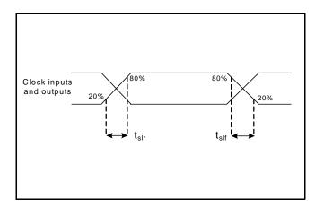
Figure 5: Input and Output Slew Rates
