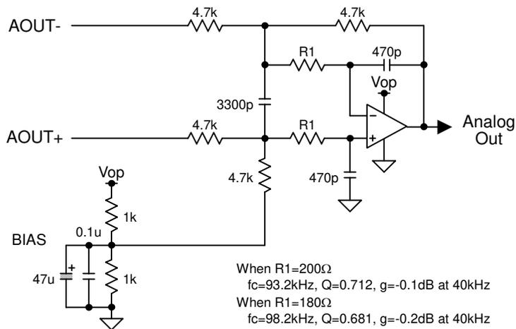
Figure 10. External 2<sup>nd</sup> order LPF Circuit Example (using op-amp with single power supply)
