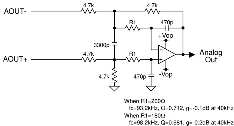
Figure 11. External 2<sup>nd</sup> order LPF Circuit Example (using op-amp with dual power supplies)
