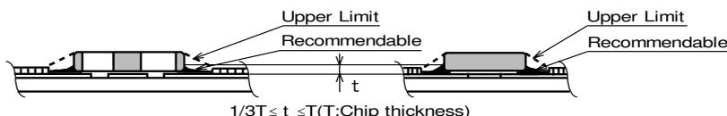
Accordingly increasing the solder volume, the mechanical stress to product is also increased.
