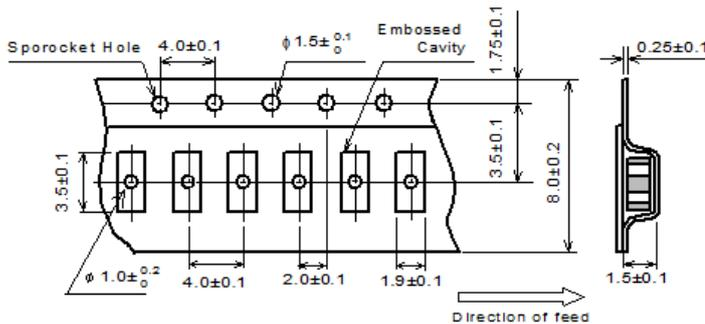
Dimension of the Cavity is measured at the bottom
