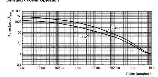
Maximum pulse load, single pulse; applicable if  $\bar{P} \to 0$  and n  $\leq$  1000 and  $\hat{U} \leq$  4 kV; for permissible resistance change equivalent to 8000 h operation in power operation mode.
