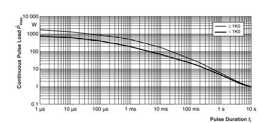
Maximum pulse load, continuous pulses; applicable if  $\bar{P} \leq P$  ( $\vartheta_{amb}$ ) and  $\hat{U} \leq 4$  kV; for permissible resistance change equivalent to 8000 h operation in power operation mode.
