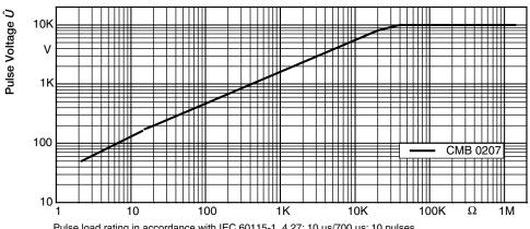
Pulse load rating in accordance with IEC 60115-1, 4.27; 10  $\mu$ s/700  $\mu$ s; 10 pulses at 1 min intervals; for permissible resistance change 0.5 %  $\pm$  (0.5 % R + 0.05  $\Omega$ ) Resistance Value R
