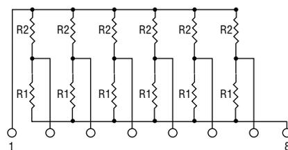
The 4608X-104 (shown above) is an 8-pin configuration and terminates 6 lines. Pins 1 and 8 are common for ground and power, respectively. Twelve thick-film resistors are paired in series between the common lines (pins 1 and 8).
