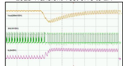
Load Transient Test 0.15 to 2A
