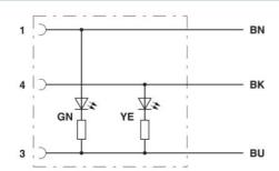
Contact assignment of M12 sockets with LED
