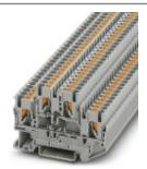
Component terminal block, with integrated 1N4007 diode, nom. voltage: 500 V, nominal current: 0.5 A, connection method: Push-in connection, number of connections: 4, cross section:0.14 mm² - 4 mm², AWG: 26 - 12, width: 5.2 mm, color: gray, mounting type: NS 35/7,5, NS 35/15
