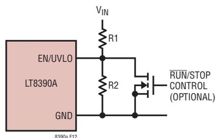
Figure 12. V<sub>IN</sub> Undervoltage Lockout (UVLO)
