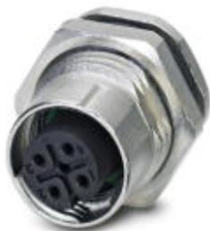
Sensor/actuator flush-type socket, 4-pos., M12 SPEEDCON, shielded, A-coded, rear/screw mounting with M12 thread, with straight solder connection
