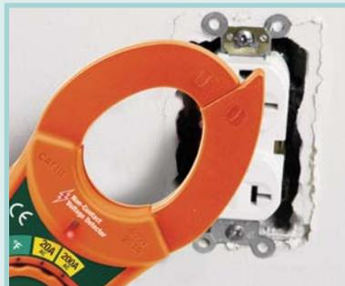
Built-in non-contact Voltage detector with LED alert
