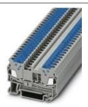
Fast connection terminal block, Connection method: Quick connection, Cross section: 0.25 mm² - 1.5 mm², AWG: 24 - 16, Width: 5.2 mm, Color: gray, Mounting type: NS 35/7,5, NS 35/15
