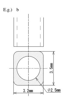
\*Nozzle with chamfering is recommended
