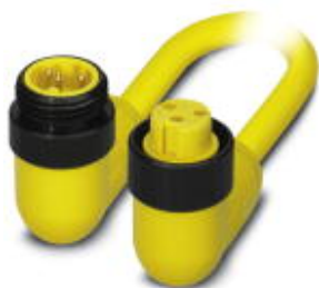
Power cable, 3-position, PVC, yellow, Plug angled 7/8"-16UNF, A - standard, on Socket angled 7/8"-16UNF, cable length: 10 m
