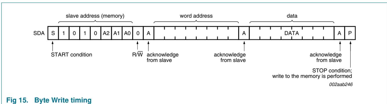
Fig 15. Byte Write timing
