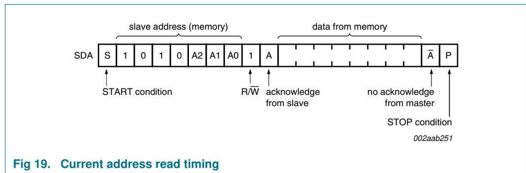
**Fig 19. Current address read timing**
