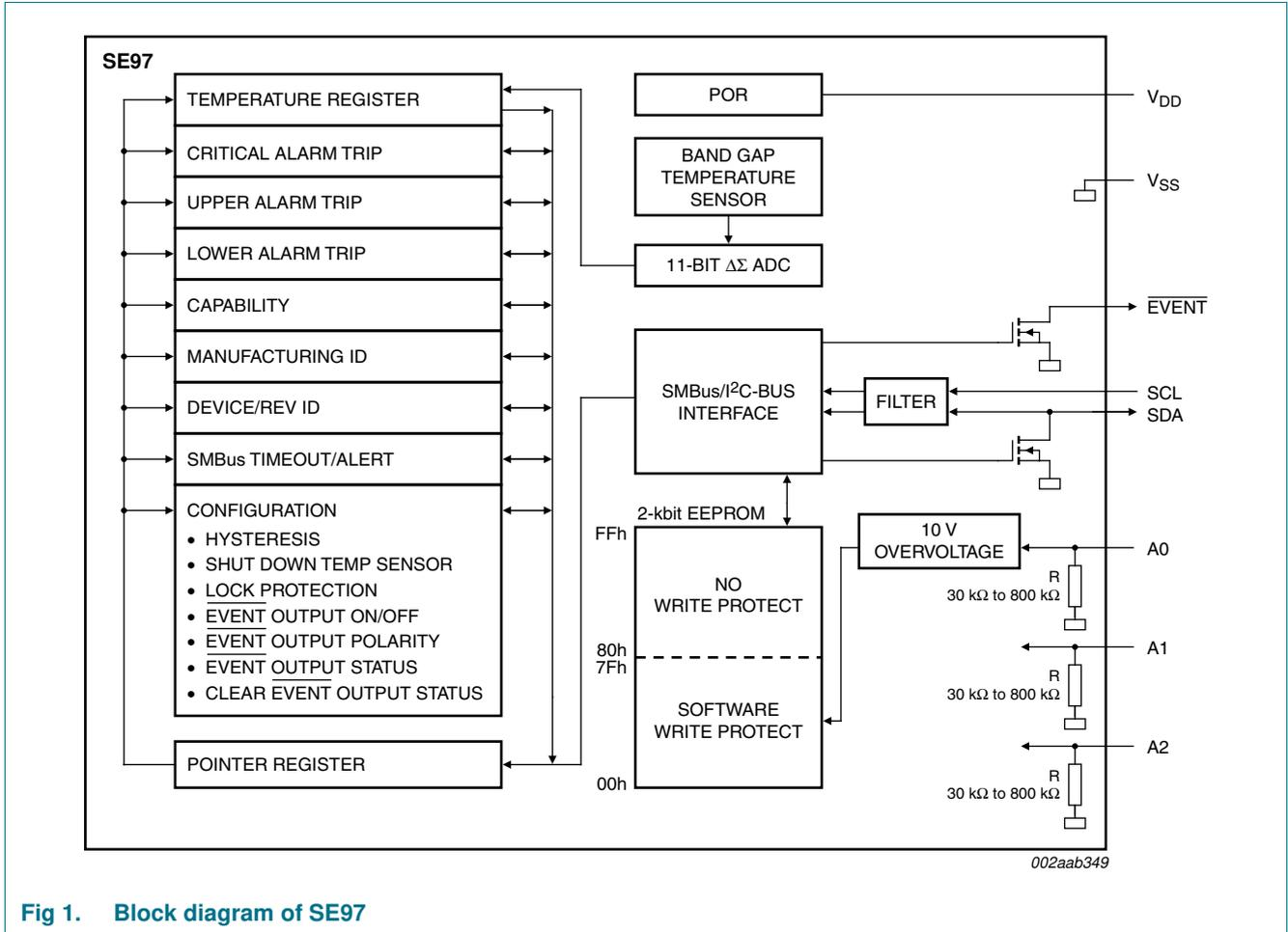
Fig 1. Block diagram of SE97
