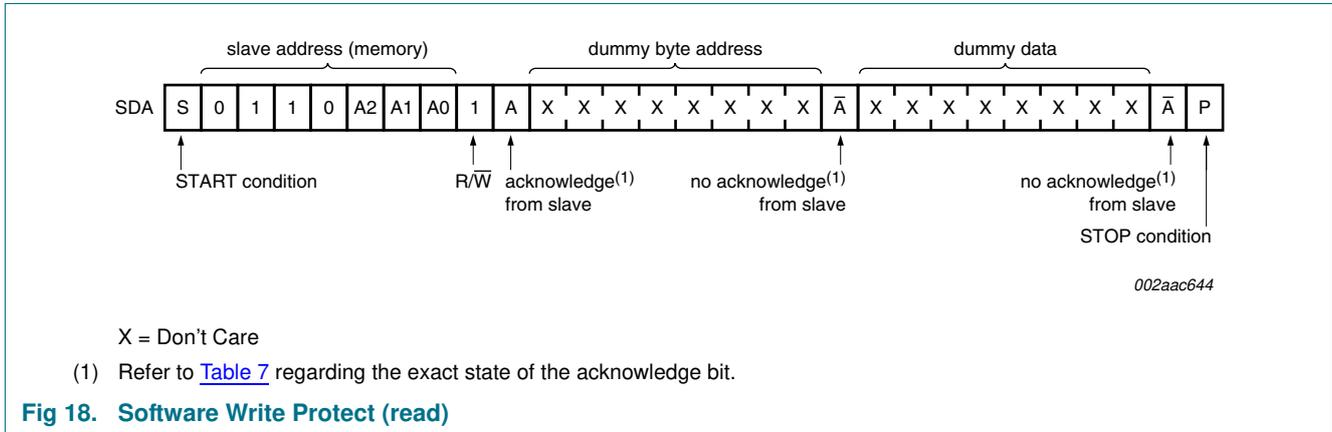
Fig 18. Software Write Protect (read)
