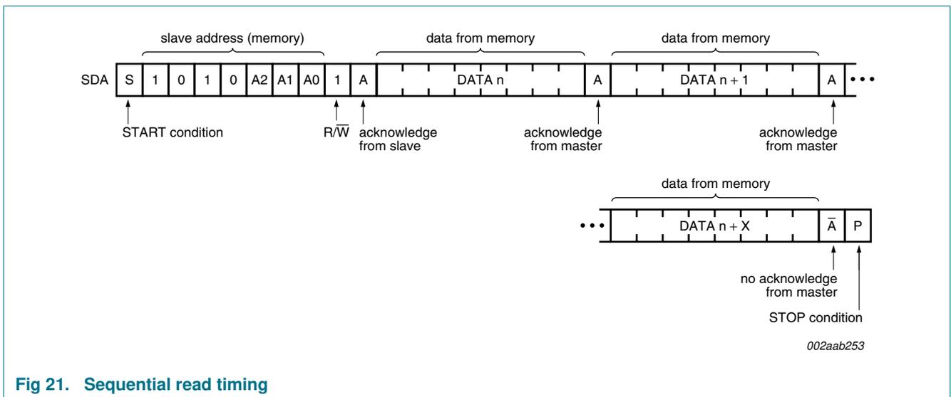
Fig 21. Sequential read timing
