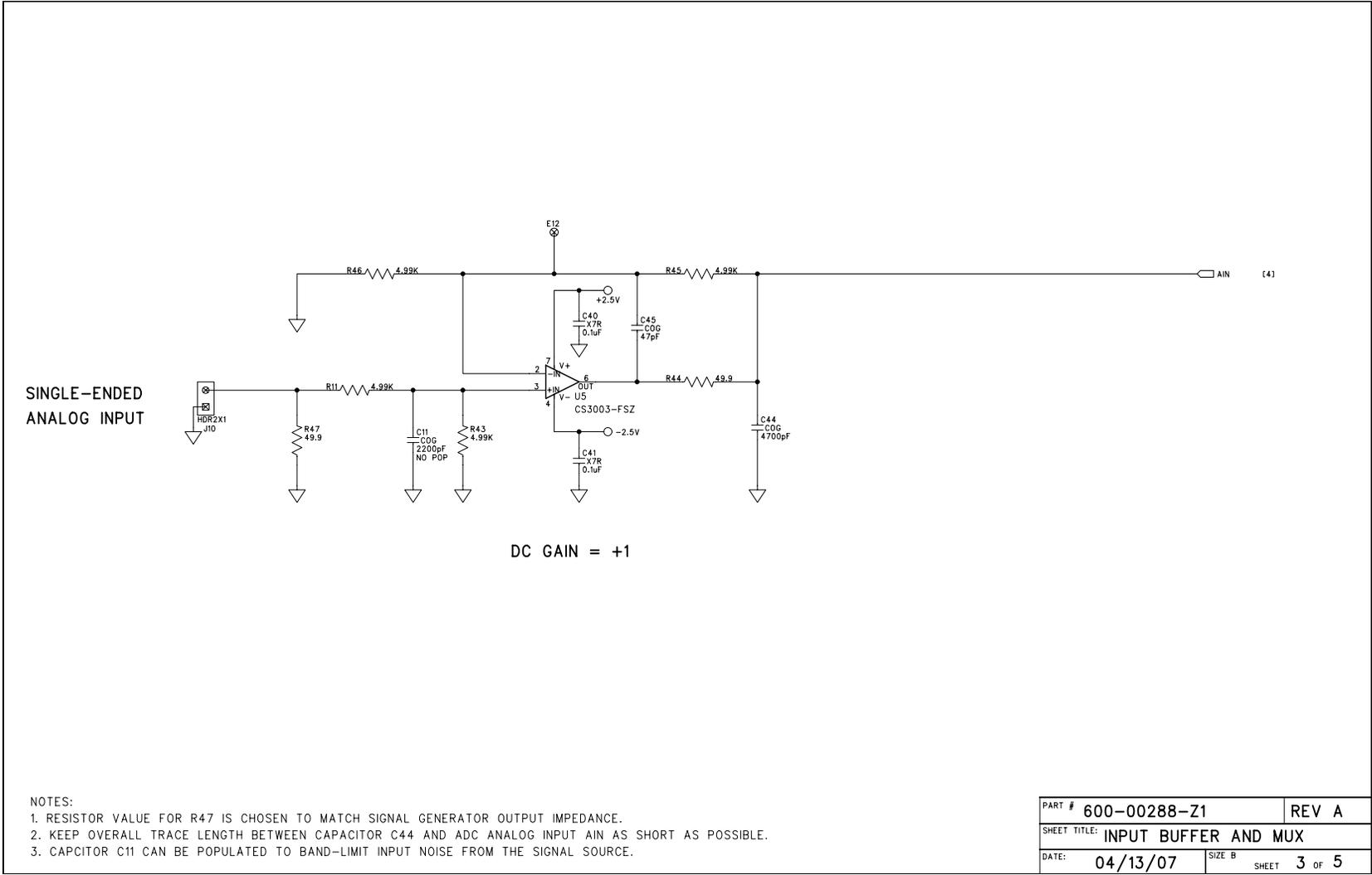
Figure 5. Schematic - Input Buffers and Multiplexer
