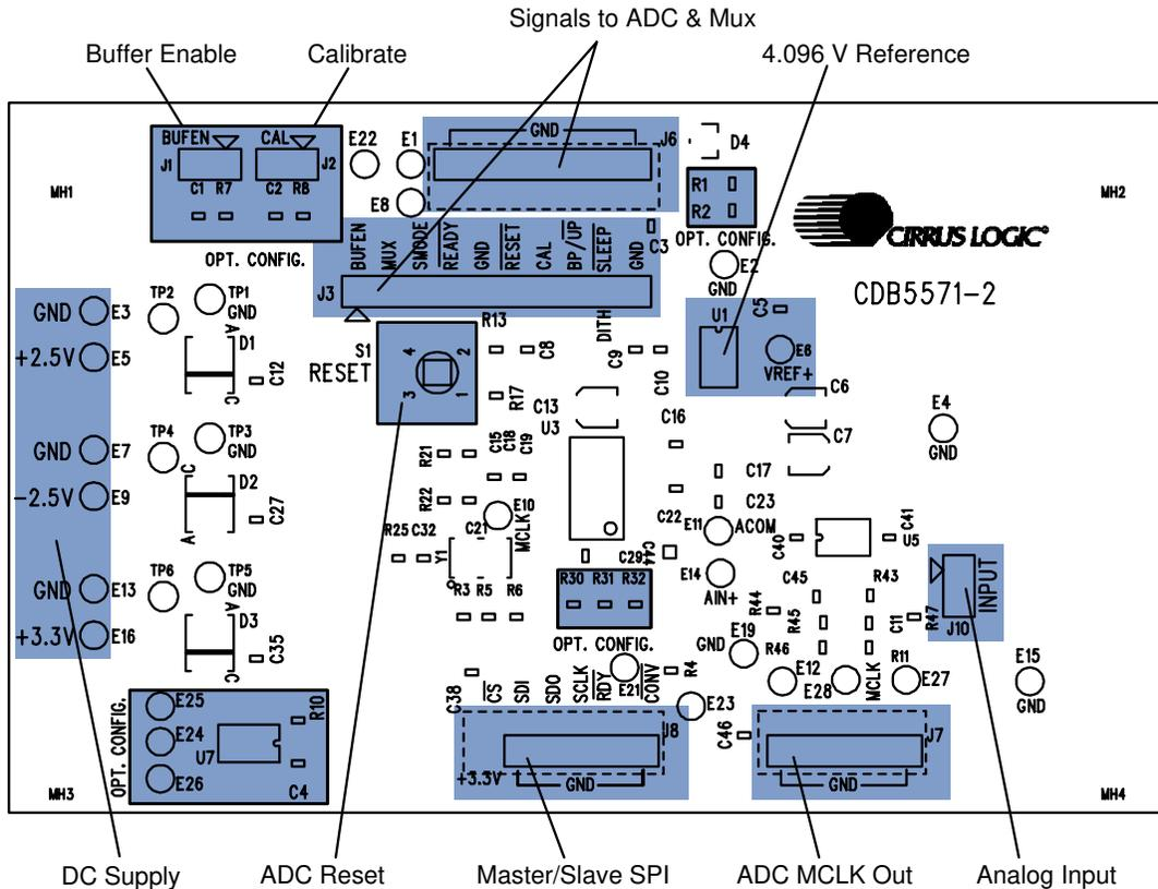
NOTE: Shaded boxes marked with "OPT. CONFIG." are not necessary for operation in an end user product.
