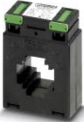
Window-type current transformer, 200 A AC primary current; 5 A AC secondary current; accuracy class 1; 7.5 VA rated power
